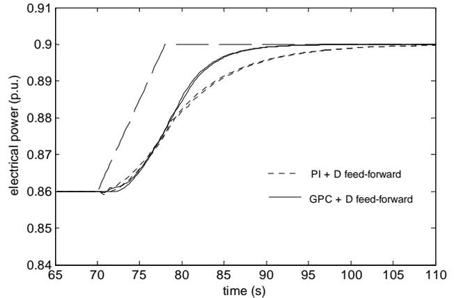
Figure 9 Comparison of the responses for the PI and CGPC designs when the derivative feed-forward loop is included (1-Unit operational case).
