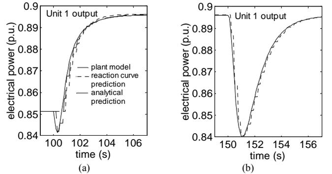
Figure 4 Response of the Plant model and the predictive models to a 0.04 p.u. step in control (U), (a) applied to Unit 1, with the controls for Units 2-6 fixed at their initial values and (b) applied simultaneously to Units 2-6, with the control for Unit 1 fixed at its initial value.
