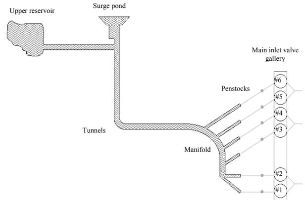
Figure 1 Schematic diagram of the tunnel and penstocks at Dinorwig (not to scale).
