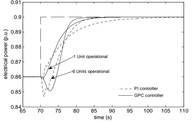
Figure 8 Comparison of the step responses produced by the CGPC design and the modified PI controller for the 1-Unit and 6-Unit operational cases.
