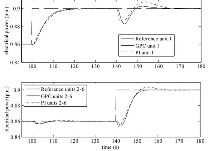
Figure 6 Responses of unconstrained GPC and PI to 0.04 p.u. step power demand for Unit 1 (upper) and Units 2 - 6 (lower).
