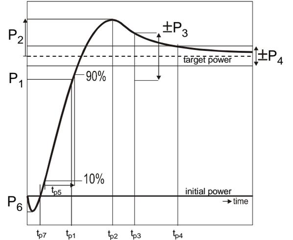
Figure 3 Specifications for a response to a step change in demanded power.
