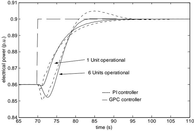
Figure 5 Comparison of the step responses produced by the GPC design and the standard PI controller for the 1-Unit and 6-Unit operational cases.
