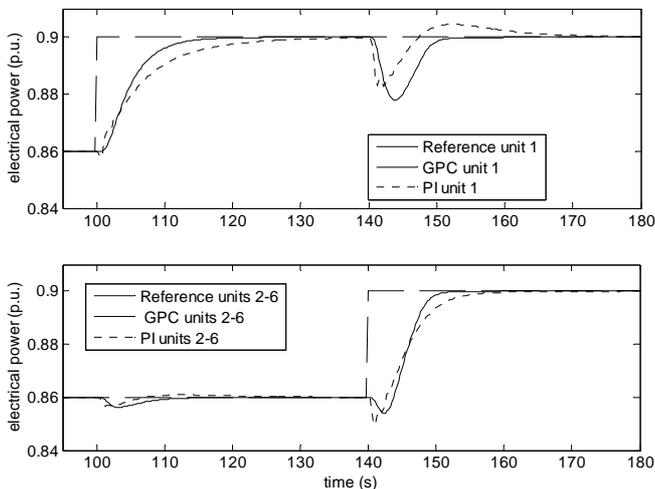
Figure 10 Responses of constrained GPC and PI to 0.04 p.u. step power demand for Unit 1 (upper) and Units 2 - 6 (lower)
