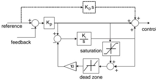
Figure 7 Anti-windup configuration for the modified PI controller, also showing the derivative feed-forward path.
