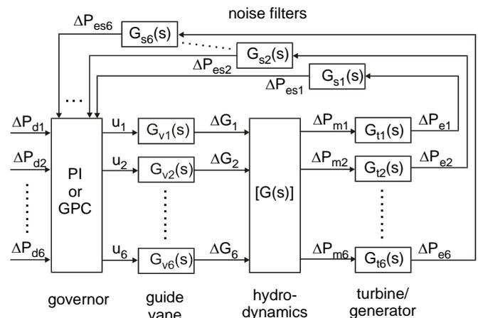
Figure 2 MIMO model of the hydroelectric plant.
