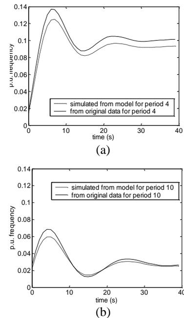
Figure 13 The step responses of 2 models identified from simulations having different input and noise sequences to the data used to identify the original model.
