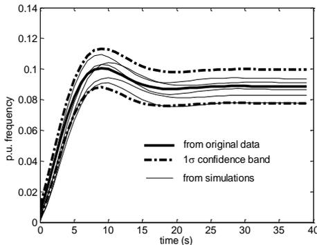
Figure 11 Comparison of the step responses of 5 models identified from simulations with different input sequences and the model identified from the original data.
