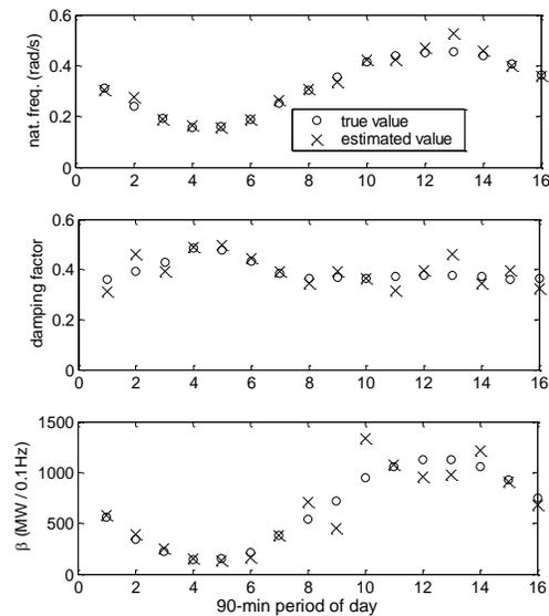
Figure 15 Simulation results comparing the values of the parameters estimated in the presence of noise with their true values.
