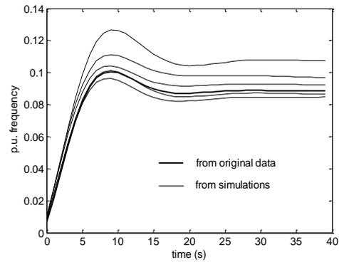
Figure 12 Comparison of the step responses of 5 models identified from simulations with different noise sequences and the model identified from the original data.
