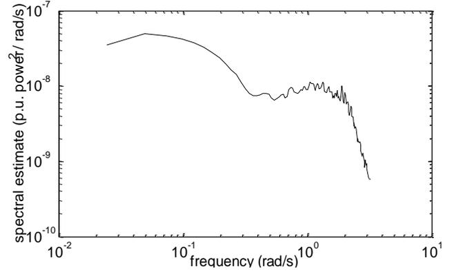
Figure 9 Spectrum of (differenced) power input  $\Delta P_e$  from Dinorwig for Dec 1<sup>st</sup> 2001.
