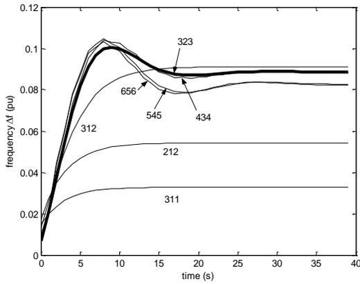
Figure 6 Response of frequency to a unit step in per-unit power for ARIMAX models of various order.
