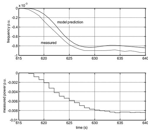
Figure 10 Comparison of measured frequency with the prediction made by the identified model.
