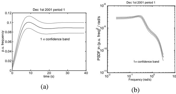
Figure 8 ARIMAX model for Dec 1<sup>st</sup> 2001, period 1 (a) step response of input-output model, (b) spectrum of disturbance model (differenced data).
