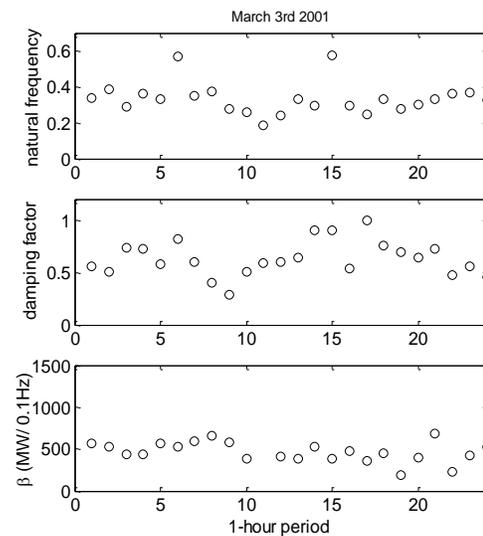
Figure 16 Daily variation of the power system's natural frequency, damping factor and stiffness over a 24 hour period.
