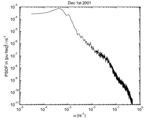
Figure 2 Spectrum of the grid frequency variation for Dec 1<sup>st</sup> 2001.
