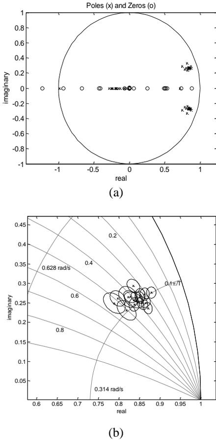
Figure 7 (a) Pole zero map for the ARIMAX323 models for sixteen 90-minute periods on Dec 1<sup>st</sup> 2001, (b) the  $1\sigma$  confidence limits for the pole locations.
