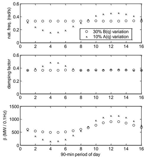
Figure 14 Zero-noise simulation to show the effect of varying  $A(q)$  by  $\pm 10\%$  and  $B(q)$  by  $\pm 30\%$ .
