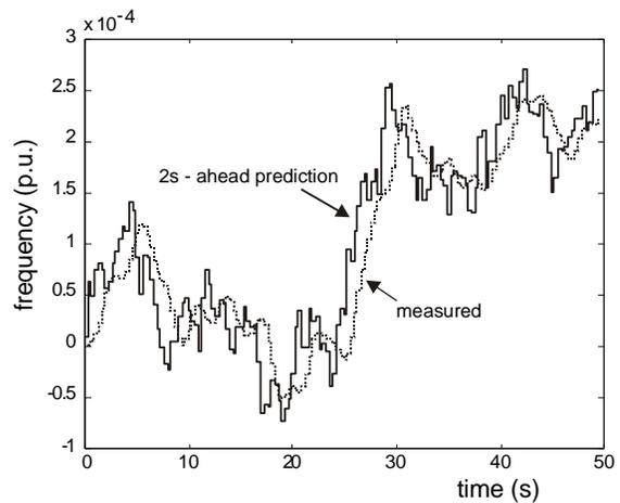
Fig. 11 Comparison of 2s-ahead predicted frequency with measured frequency.
