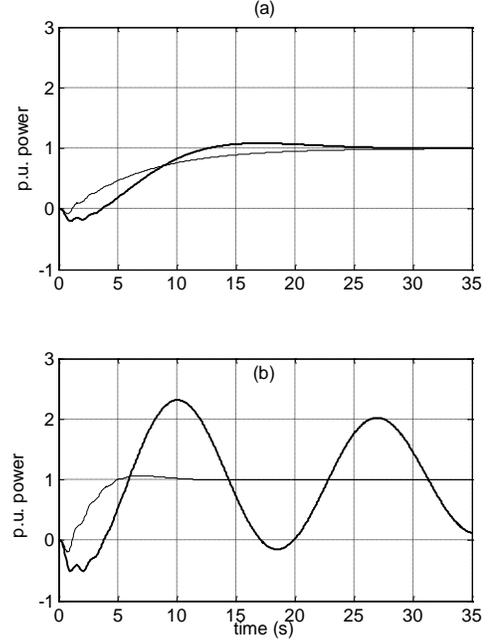
Fig. 5 Comparison of closed loop power generated in response to an unit step increase in Grid load for (a)  $K_p = 10$ ,  $K_i = 12$ ,  $K_d = 2$  (b)  $K_p = 24$ ,  $K_i = 28.8$ ,  $K_d = 2$  where the thick lines denote  $T_W = 2.7s$  (6 Unit operation) and the thin lines denote  $T_W = 0.7s$  (1 Unit operation).
