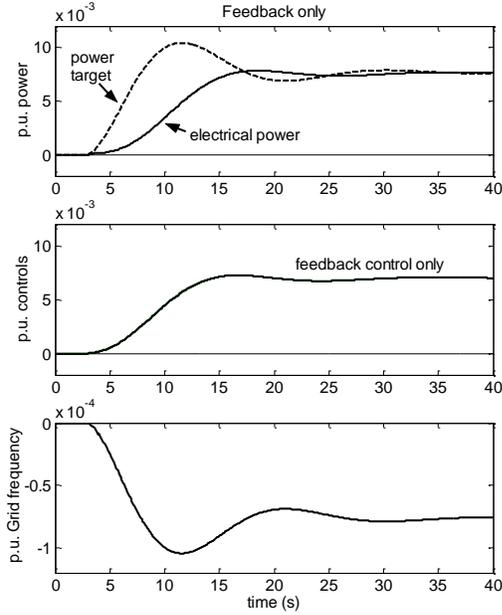
Fig. 6 Response to a step increase in Grid load at  $t = 3$ s with feedback control only, (a) generated and target power, (b) controls, (c) Grid frequency.
