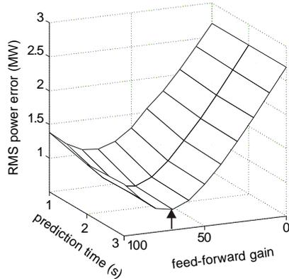
Fig. 13 RMS value of power error as a function of the prediction time and feed-forward gain; the arrow shows the minimum error over the range of values considered.
