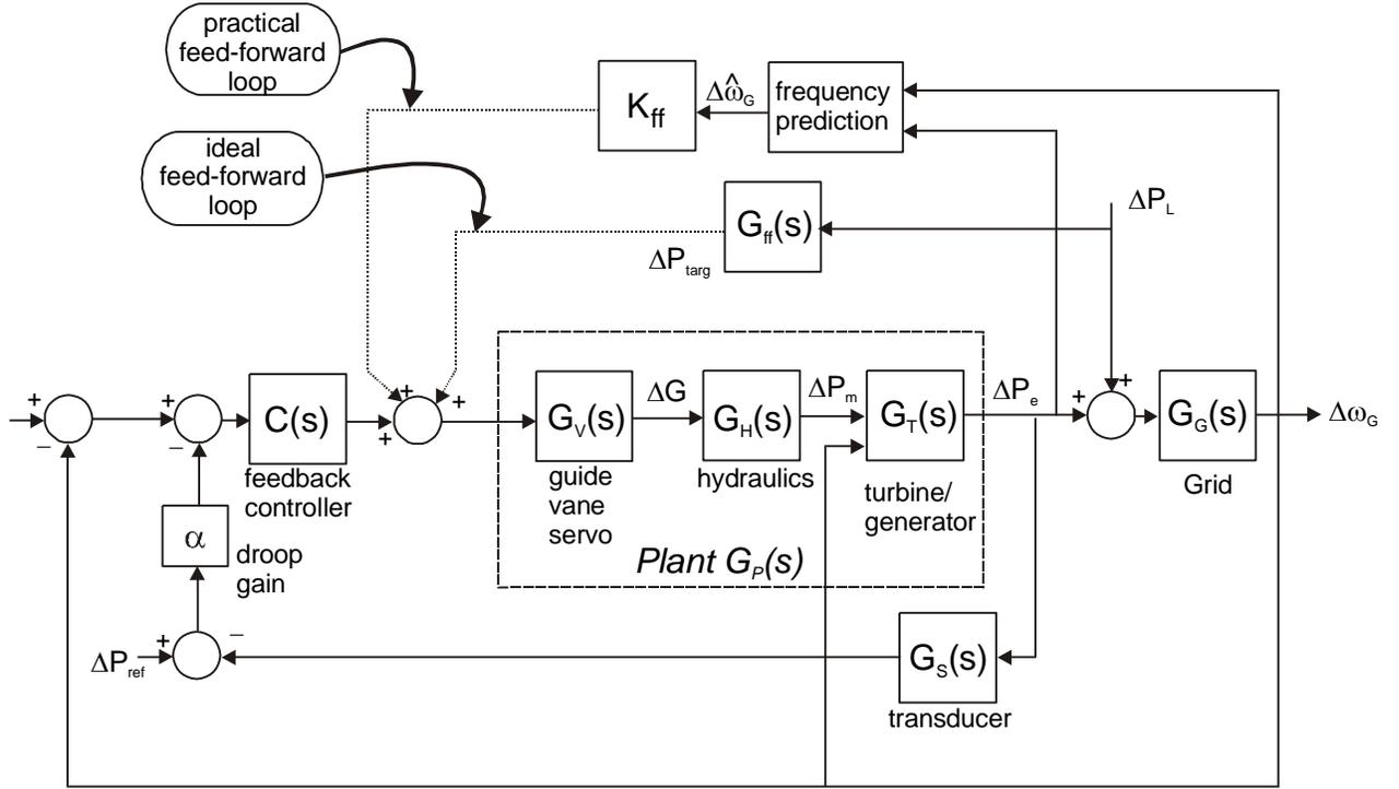
Fig.1 Block diagram of the linearised system model for one turbine/generator operating in PLR mode.
