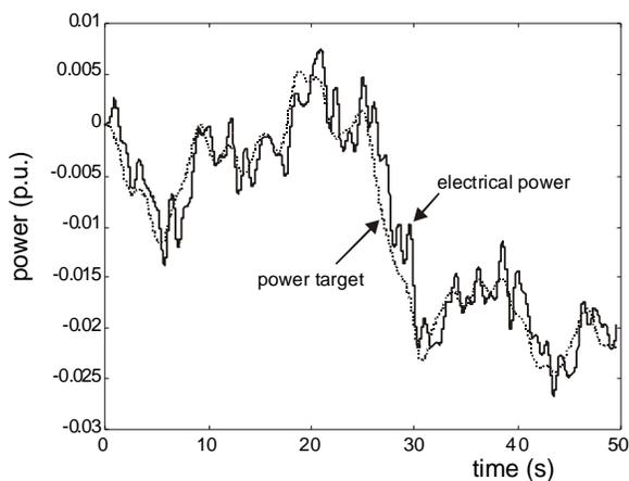
Fig. 10 Tracking of electrical power to its target, FF gain = 65 and 2s-ahead prediction.
