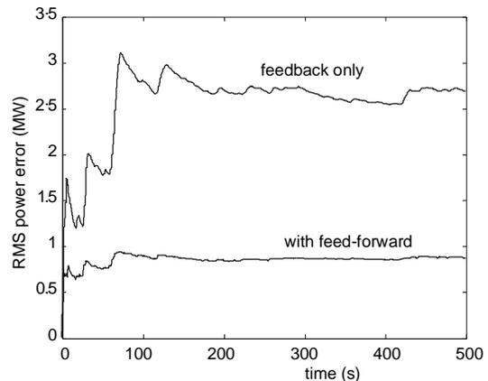
Fig. 12 RMS value of the error between the power delivered and the power target.
