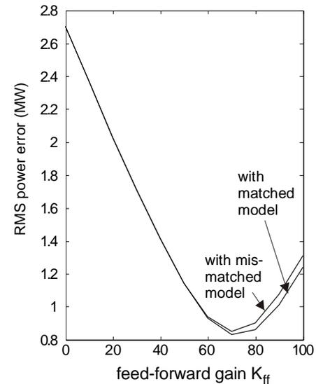
Fig. 15 Effect of mis-match between predictor model and actual system on the rms power error, as a function of feed-forward gain.
