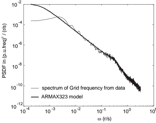
Fig. 4 Power spectral density function of the Grid frequency record of Fig. 2 and the model identified from the data.
