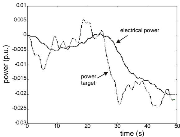
Fig. 9 Tracking of electrical power to its target, FF gain = 0.
