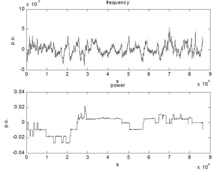
Fig. 2 Record of per-unit Grid frequency and total power flowing at Dinorwig for the 24-hour period of 4<sup>th</sup> March 2001.
