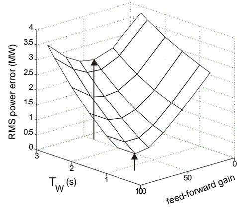
Fig. 14 RMS value of power error as a function of the water starting time and feed-forward gain. The minima for  $T_w = 2.7s$  (large arrow) and  $T_w = 0.7s$  (small arrow) are shown.
