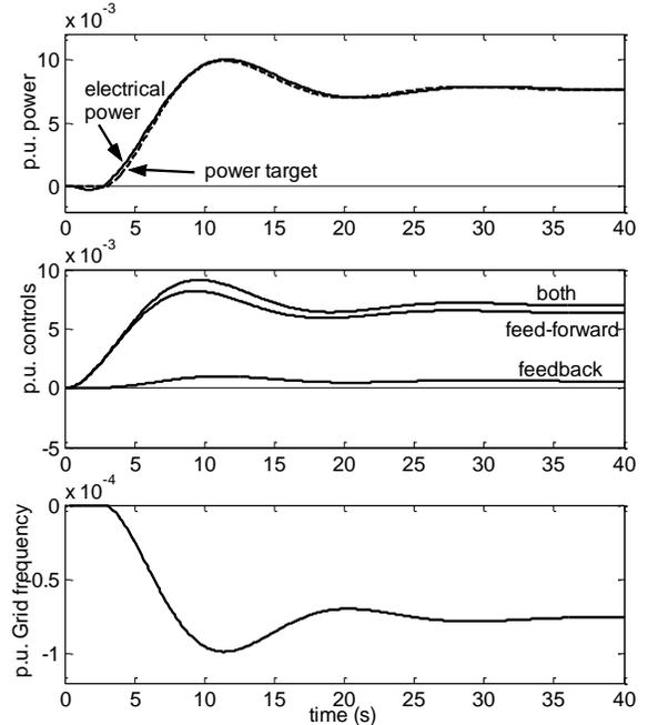
Fig. 7 Response to a step increase in Grid load with both feedback and feed-forward control, (a) generated and target power, (b) controls, (c) Grid frequency.
