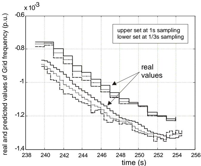
Fig. 8 Comparison of j-step-ahead predictions for 1s and 1/3s sampling rates.
