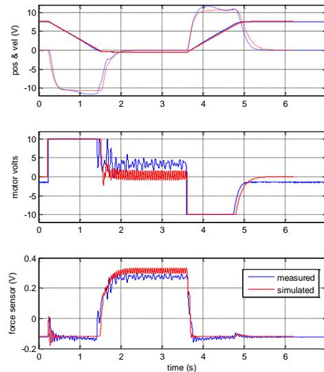
Fig. 9 Simulated and measured responses showing deployment, contact with the OHL and retraction. Values of  $B = 0.82$ ,  $\dot{\theta}_o = 0.56\pi$ ,  $F_c = 0.27N$  and  $m/M = 75$  were used, which are very close to the prototype values.
