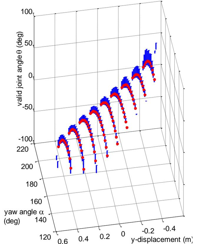
Fig. 5 Ranges of valid joint angle ( $\theta$ ) as a function of roll angle, yaw angle and lateral displacement.
