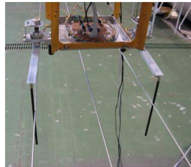
Fig. 11 The pick-up mechanism during contact with the OHL.
