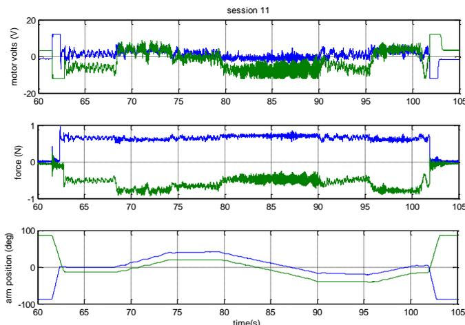
Fig. 10 Result from an AVS test showing the servomotor voltages, sensor forces and link positions.
