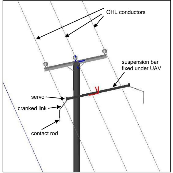
Fig. 2. Output of a Matlab 3D visualization program showing the pick-up mechanism relative to the OHL.
