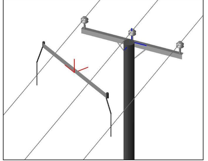
Fig. 4 Example of pick-up mechanism configuration to compensate for simultaneous yaw and lateral displacement of the suspension.
