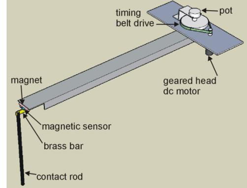
Fig. 7 Construction of the pick-up mechanism.
