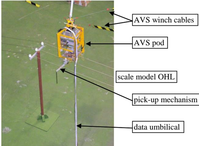
Fig. 6 Photograph of the AVS pod ‘flying’ above the model power lines; the experimental pick-up mechanism is fixed underneath, with links retracted.
