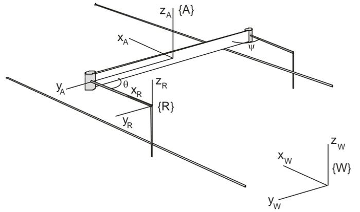
Fig. 3. Frames of reference for the 3D visualization program.
