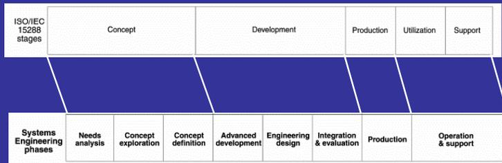
Each succeeding phase adds a further level of requirements or specifications to serve as a basis for the next phase. Each phase produces an increasingly detailed definition ('materialisation') of the system until the final product or service has been achieved.
