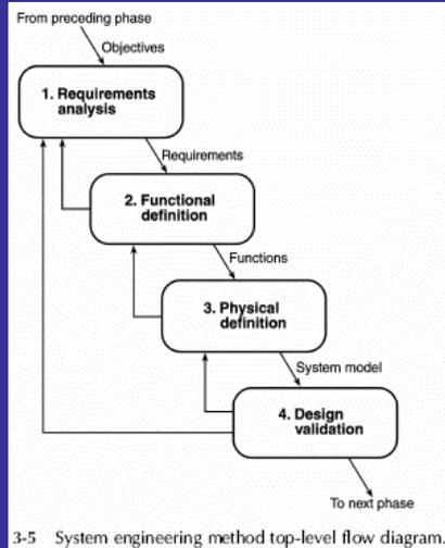
3-5 System engineering method top-level flow diagram.
